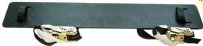
Boom Guard (24-03GUARD) Protects boom from saw damage. Mount on boom in front of tool holder to avoid damaging boom when inserting tool into holder. 32" X 5"
